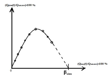
The method of straight line is based on the dependence of the change in time of the annual gas production in the period of decline whih is described by exponential function in such form
