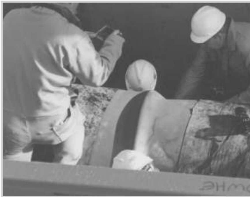
Fig. 9—8. Pipeline buckle caused by differential settlement through a landfill (Source: National Transportation Safety Board)
