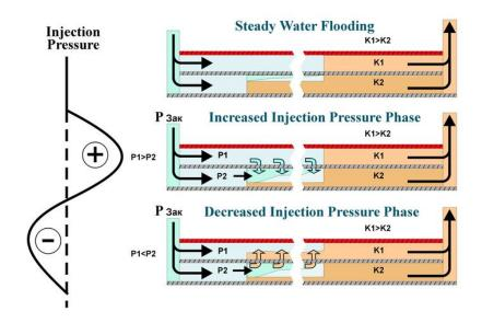
Figure 5.2 – Dynamics of pressure change during cyclic flooding
