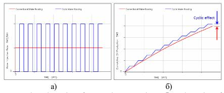
a) – dunamics of pumped water volume  $\boldsymbol{6})$  – dynamics of accumulated production
