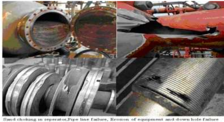
Figure 1 – Sand choking in separator, pipe line failure and other problems with sand flow.
