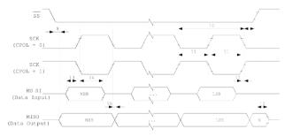
In principle, the timings are the same in slave mode like previously described in master mode. Because of the switching of the roles between master and slave the requirements on the timing are inverted as well. The minimum times of the master mode are now maximum times and vice versa.
