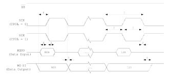
The minimum timing of the clock signal is given by the times "1" and "2". The value "1" specifies the SCK period while the value "2" specifies the high / low times of the clock signal. The maximum rise and fall time of the SCK signal is specified by the time "3". These are the first timings of the AVR to check if they match the requirements of the slave.
