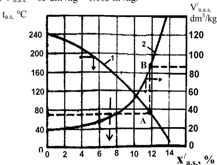
**Figure 2.1** – The figure for determination of the increase of the temperature of acid solution and the norm of flow rate of acid (15 % concentration) per 1 kg of magnesium
