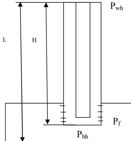
**Figure 1.1** – Figure for determination of the wellhead pressure during the completion of gas well (completion by the method of replacing the liquid that is replacing the drilling mud by gas condensate).
