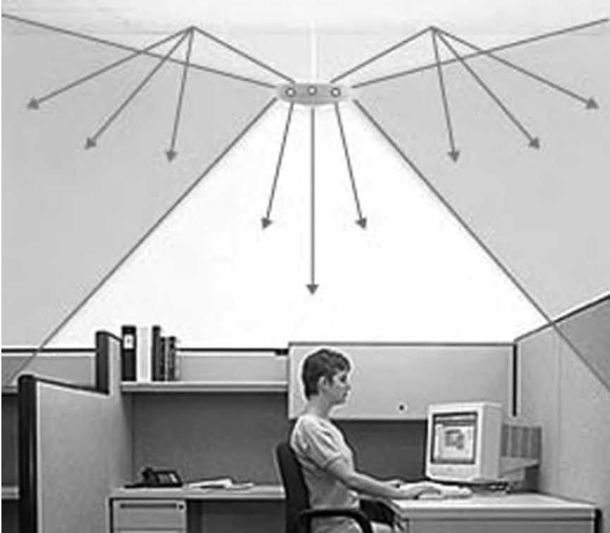
Figure 5-25. Up-Down Light Fixture
